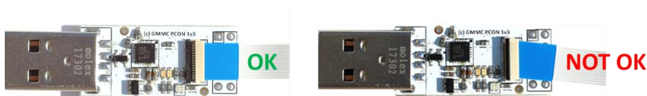
Figure 2 Kit modules interconnection via FFC cables
