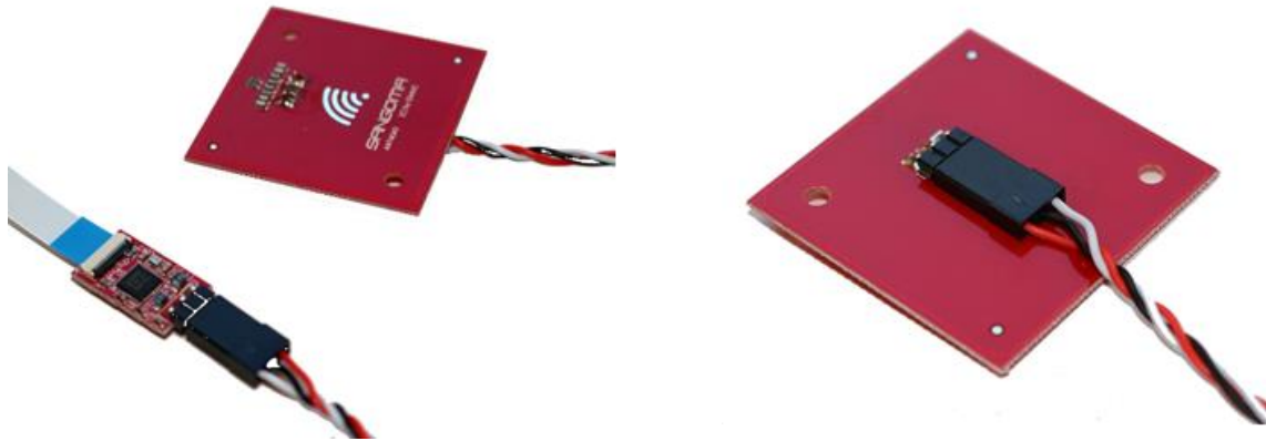
Fig 8 NFC Module antenna connection
